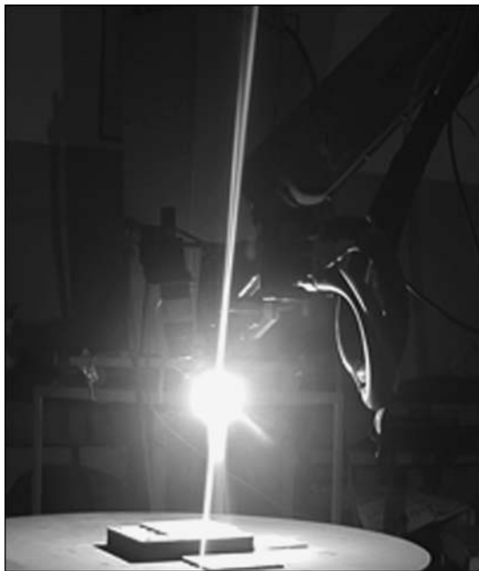
Fig. 2 Experimental setup with the pyrometer and plasma torch on the same robot arm
